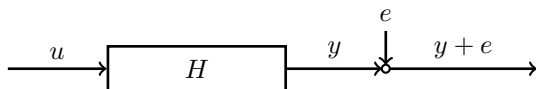
Fig. 2. System H maps any input u \in \mathcal{U} to the corresponding output y . The measured output is corrupted by measurement noise e .
