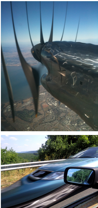
Fig. 1. Distortion effects caused by rolling shutter [2]
