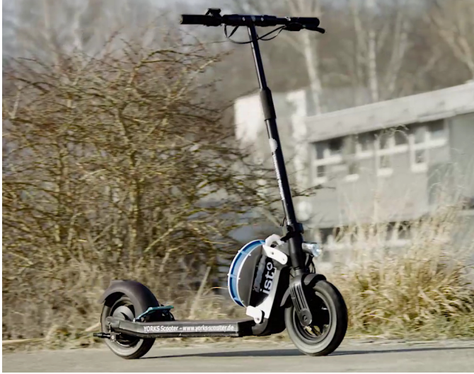
Fig. 1. The first prototype of the self-balancing e-scooter driving without a person. The reaction wheel used to balance the scooter is mounted in the blue cylinder.
